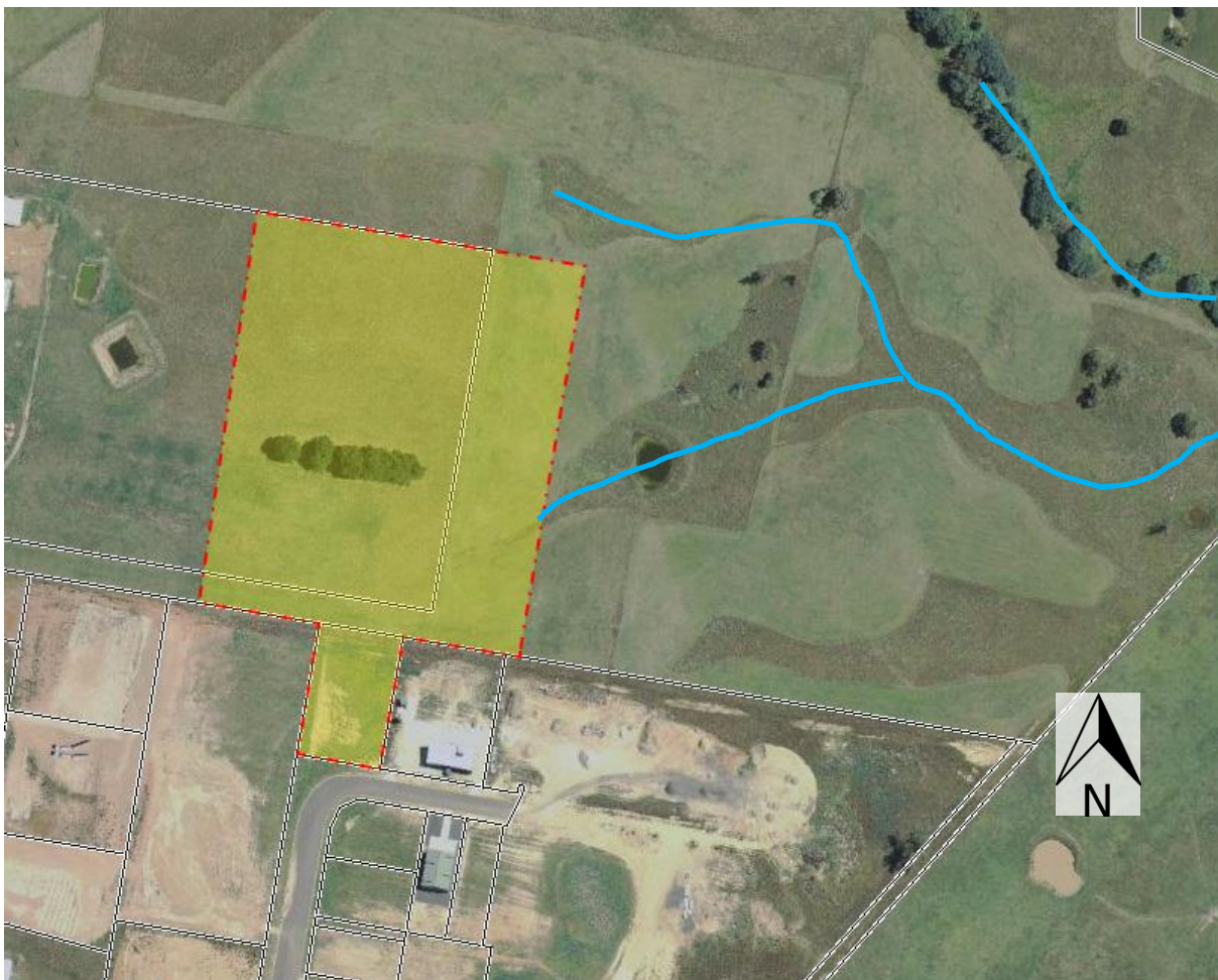
Figure 2 Overland flow paths (not creeks as defined in the Water Management Act) adjacent to Lot 34.
